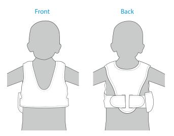
2 Place the vest over the head. The rear section should lie between the shoulder blades.
